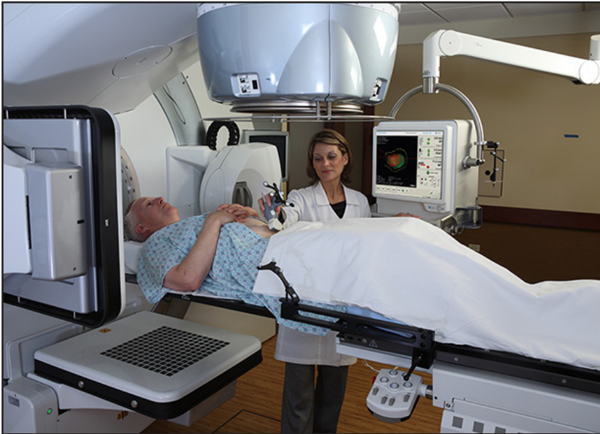
Hybrid imaging is achieved by acquiring Elekta's Clarity images at the same time as the CT acquisition procedure with the patient in the same RT setup position. This allows CT and Clarity images to be automatically fused for seamless integration into simulation and planning workflows. Clarity's software-assisted segmentation technology supports clinicians in rapidly contouring 3D soft-tissue targets and anatomy prior to treatment planning.
