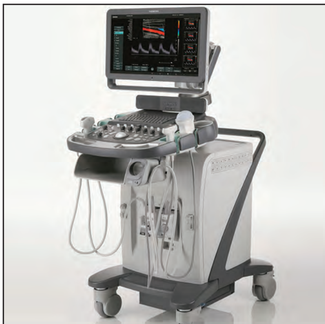
FIGURE 5. The 2.0 release of Siemens' Acuson X700 includes eSie Touch elasticity imaging for noninvasive tissue stiffness analysis.
