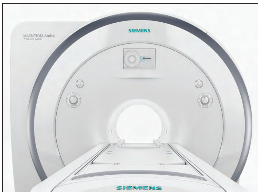
FIGURE 11. Siemens' MAGNETOM Amira features the 510(k) pending SEEit MR application for noninvasive prostate MR exams without an endorectal coil.
