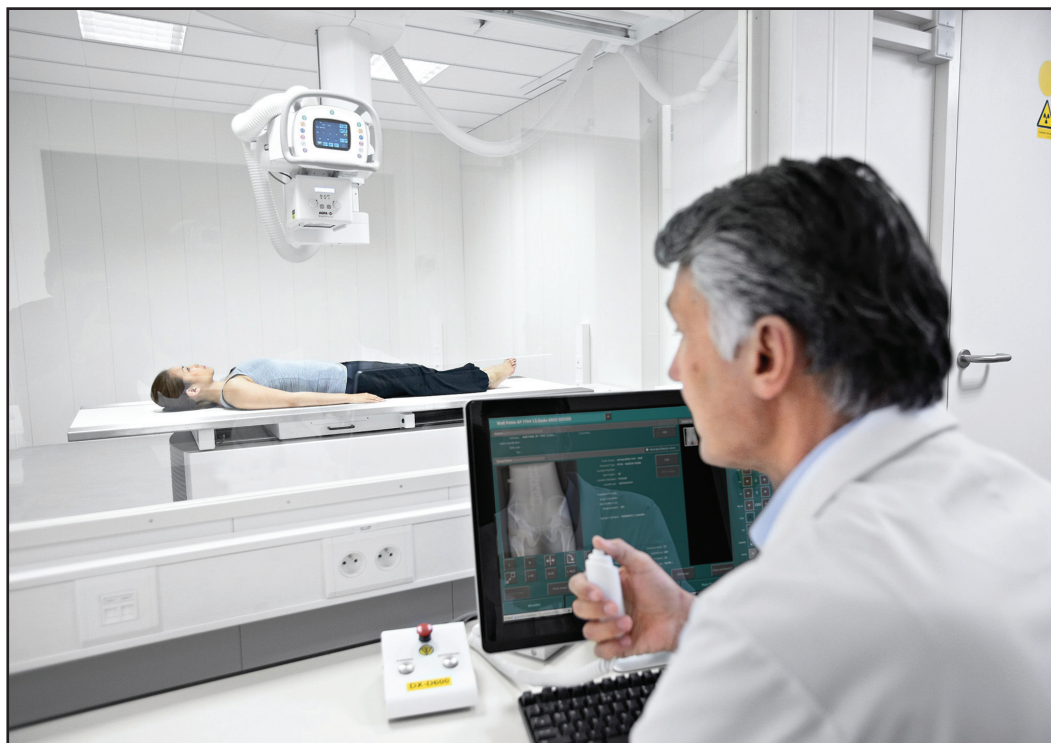
Agfa DR 600 multi-detector system features ZeroForce Technology for manual movement of the tube head in all directions with minimal effort.
