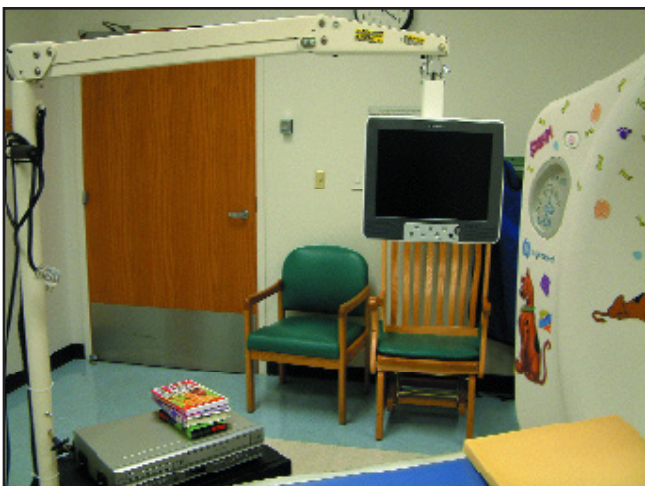
FIGURE 3. A DVD player with a flat-screen monitor on a multijointed arm. With a multijointed arm, the screen can be positioned in the child's view regardless of how the child is positioned in the CT gantry.
