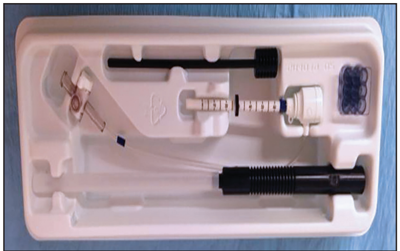
FIGURE 4. MRI biopsy kit with a coaxial system (ATEC Introducer Localization Set, Hologic, Bedford, MA). Top center: Plastic obturator inner component. Top right: Needle guide. Middle row, center: Outer component of the coaxial system with the introducer sheath, which has depth graduations and a mobile depth marker. Bottom row: Metallic, cutting introducer stylet inner component.
