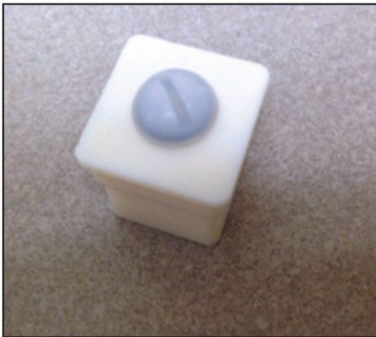
FIGURE 3. Fiducial marker (Invivo Corp.) placed within the grid helps with targeting and orientation, appearing hyper-intense on T1-weighted sequences.
