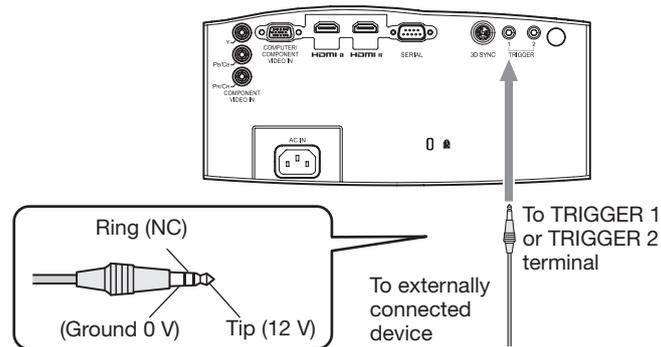
To use the TRIGGER terminals, set TRIGGER 1 (POWER) or TRIGGER 2 (ANAMO) to ON in the INSTALLATION menu. (The factory default is OFF. See page 32 for details.) Use the following steps to change the setting.
