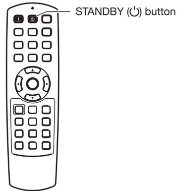
9. Press the POWER button on the projector or the STANDBY (⏻) button on the remote control.
