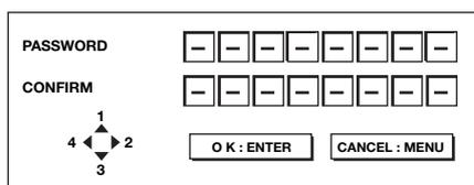
6. Enter a 4 - 8 digit password using the ▲, ►, ▼ or ◀ buttons on the remote control as shown below. (▲=1, ►=2, ▼=3, ◀=4)
