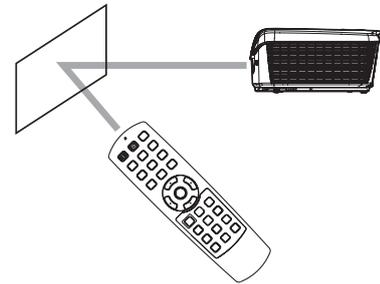
When operating the remote control, keep the distance from the remote control to the projector via the screen within about 5 m (15 feet). The operable range of the remote control, however, depends on the characteristics of the screen.
