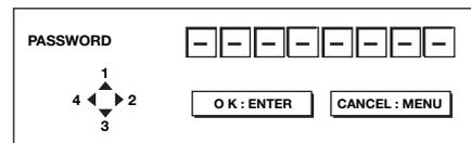
5. Enter a 4 - 8 digit password using the ▲, ►, ▼ or ◀ buttons on the remote control as shown below. (▲=1, ►=2, ▼=3, ◀=4)
