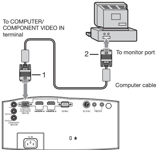
1. Connect one end of the supplied computer cable to the COMPUTER/COMPONENT VIDEO IN terminal of the projector.
