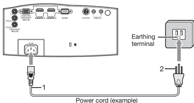
1. Plug the attached power cord into the power cord inlet of this projector.
