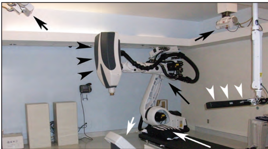
FIGURE 2. A 6-MV linear accelerator (black arrowheads) is mounted on a robotic arm (long black arrow). Diagnostic (kV) x-ray tubes (short, black arrows) are mounted on the ceiling directed toward 2 flat-panel digital imagers (short, white arrow). The patient wears a special vest (long, white arrow) that allows detection of patient motion by the nearby camera array (white arrowheads).
