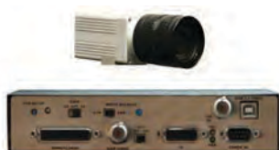
MegaRAD3 produce color or monochrome video up to 3 \times 10^6 rads total dose
