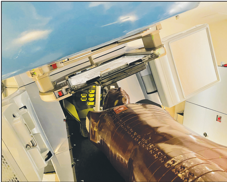
FIGURE 3. Novel configuration for electron ultrahigh dose rate radiation therapy (UHDR-RT) by No and Wu et al at Stanford University. A coneless electron applicator system is used for field shaping and to allow for closer surface-to-surface differences to achieve UHDRs, using a reversible configuration of a Varian Trilogy. An anatomical phantom is pictured on the treatment couch as a patient surrogate.
