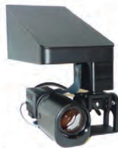
KiloRAD PTZ radiation resistant camera with Pan/Tilt/Zoom
