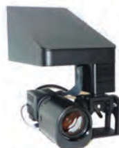
KiloRAD PTZ radiation resistant camera with Pan/Tilt/Zoom
