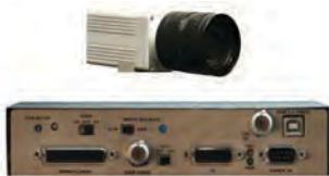
MegaRAD3 produce color or monochrome video up to 3 \times 10^6 rads total dose
