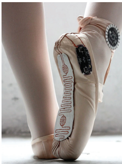
Motion tracking hardware integrated with dance costuming
