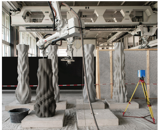
Printing concrete columns for a dance performance
